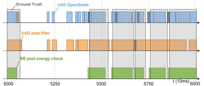
**Figure 3: Identifying voice activities. The ground truth (transparent black) from human coders is compared to voice activity detection from openSMILE (VAD, blue), VAD after applying a low-pass filter (VAD post-filter, orange), and a speaking binary classifier after performing a energy-based check to filter background noise (SB, green).**
