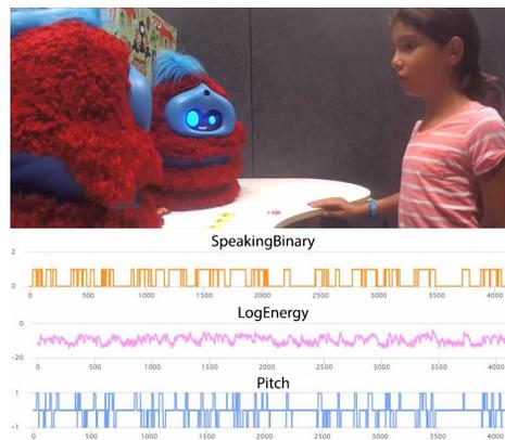
**Figure 1: We investigate the effects of an attentive listening robot on a child's storytelling behavior. The robot detects nonverbal prosodic cues from the storyteller's speech to provide backchannel feedback to signal engagement.**
