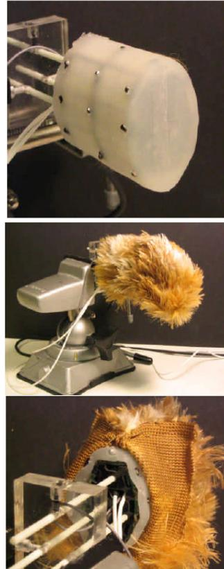
Fig. 6 The Finished Arm Test Section. At top is the silicone skin. In the middle is the completed assembly. At bottom shows the layered structure.
