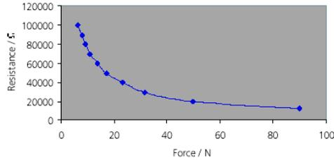
Fig. 3 The Plot of the Resistance vs. Force for the QTC Switch Substrate [14].
