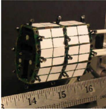
Fig. 5 The Arm Section. Each white square is one QTC sensor. The silver sensors above the surface of the QTC sensors are the thermistors. The electric field sensing electrode, not shown, is located on the bottom plane of the sensor circuit boards. All dimensions shown are in inches
