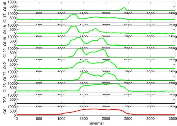
Fig. 9 The Response to Petting Motion by a Human Hand. The eight green lines are the response of the QTC sensors from one sensor circuit board. The next three black lines are the response of the temperature sensors of the same sensor circuit board. The red line at the bottom is the response of the electric field sensor.
