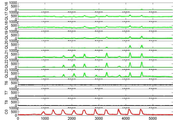
Fig. 8 The Response to a Series of Ten Pats by a Human Hand. The eight green lines are the response of the QTC sensors from one sensor circuit board. The next three black lines are the response of the temperature sensors of the same sensor circuit board. The red line at the bottom is the response of the electric field sensor.
