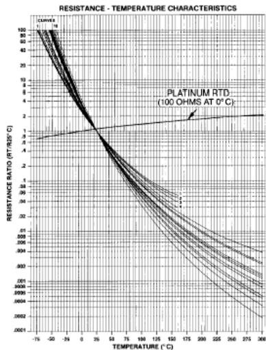
Fig. 4 Resistance Ratio vs. Temperature Characteristics for Thermistors and RTDs [15].
