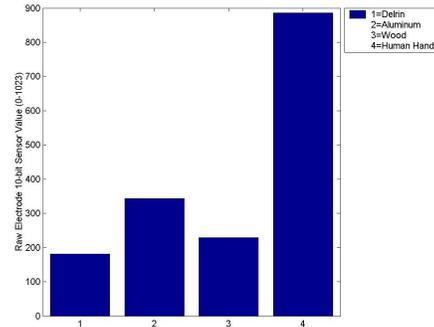
Fig. 7 The Response of the Electric Field Sensor to Contact with Delrin Bar(1), Aluminum Bar (2), Wood Bar (3), and Human Hand (4).
