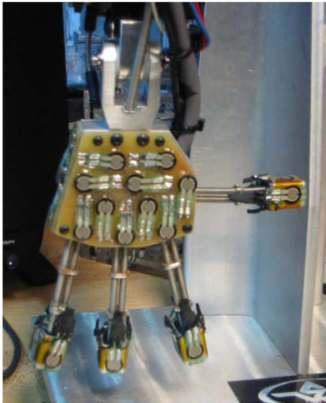
Figure 5-33. The Assembled Hand – Back of Hand View
