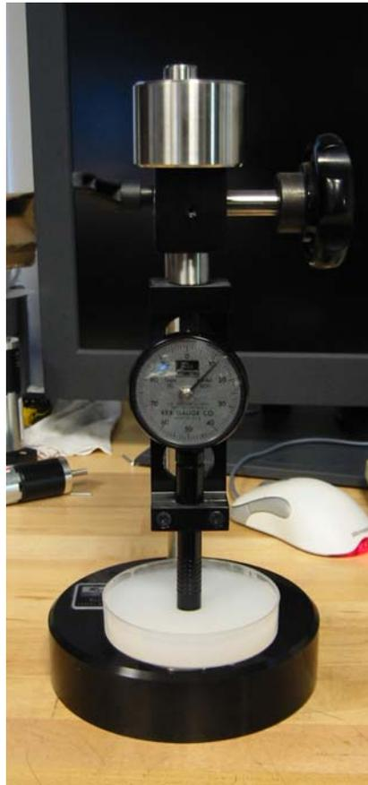
Figure 7-14. The Measurement of the Durometer of the Twelve Silicone Samples.
