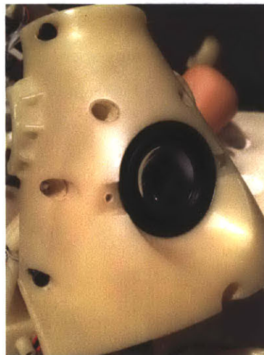
Figure 3-14: Speaker cavity in chest plate with speaker
