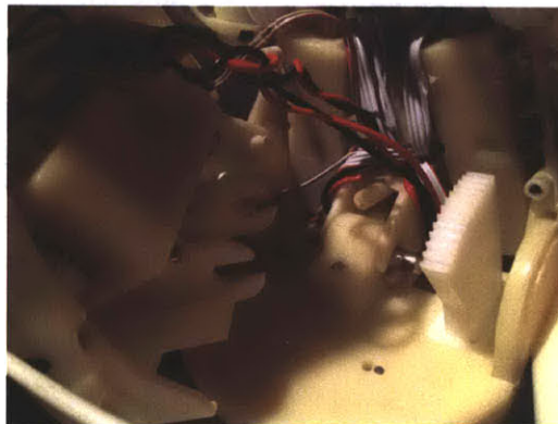
Figure 3-11: Waist bend mechanism and shaft clips for waist
