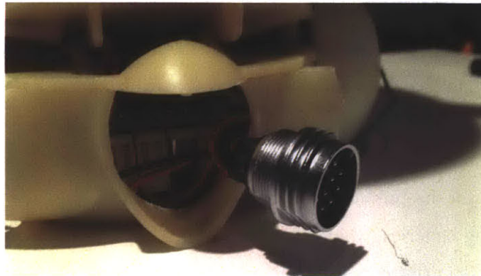
Figure 3-19: Back view of Huggable to show power port
