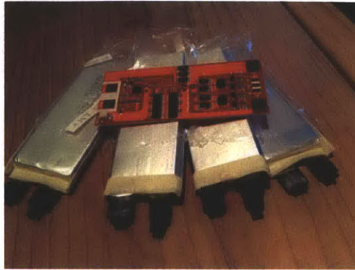
Figure 3-23: LiPo battery cells and Protection Circuit Module from Powerizer
