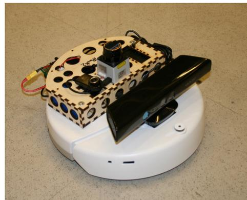
Fig. 5. The "iPuck" robot with laser scanner, Microsoft Kinect depth camera, and on-board Intel Atom PC.
