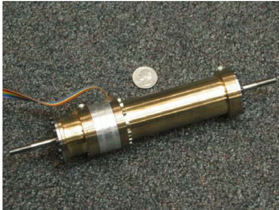
Figure 6. Self-contained electro-hydraulic actuator
