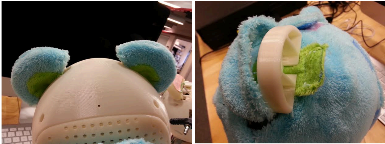
Figure 3-17. Separated ear fur piece that can be fastened with Velcro
