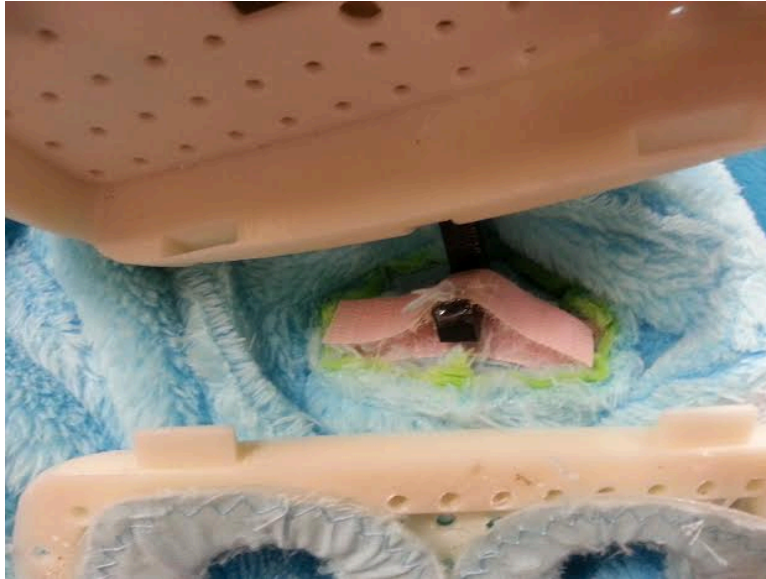
Figure 3-20. The muzzle joint stack is attached to the nose fur
