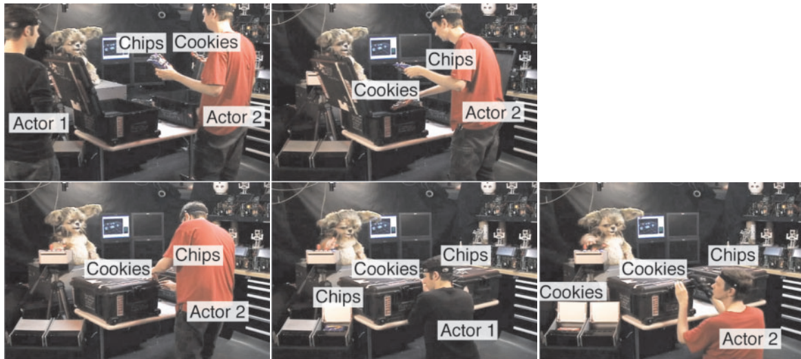
Fig. 11. Setup of the human–robot study for Tasks 4a and 4b. The scenario proceeds from upper left image to bottom right. First, actor 2 places chips in the left box and cookies in the right box for all to see. While actor 1 is absent, actor 2 switches the food items. Actor 1 returns looking for chips, but going to the wrong box. The robot realizes the false belief and invalid plan of actor 1, and gives them the chips they desire. Actor 2 (with true beliefs and a valid plan) returns looking for cookies, and the robot opens the small box revealing matching cookies. See also Extension 1.
