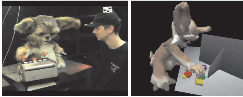
Fig. 1. Leonardo, operating a remote control panel with a slider, a button and a switch used in our cooperative behavior experiment. The robot can track objects and people tagged with reflective markers. The simulated Leonardo can perform more dexterous tasks than the physical robot, such as inserting pegs into blocks used in our social learning experiments. People demonstrate the task to be learned using a computer mouse to move objects in the virtual world.
